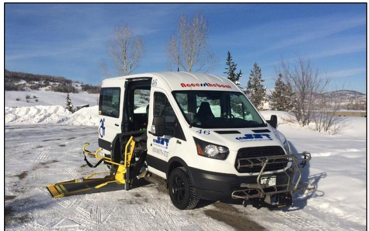
Seating is available for up to six passengers and an innovative floor design allows for unlimited securement combinations that accommodate a multitude of mobility devices from large battery-powered wheelchairs to the lightweight, wide-based sport chairs that have become popular in Steamboat Springs’ active community. Equipped with 4-wheel drive, this van is set up to handle all seasons and every condition.
