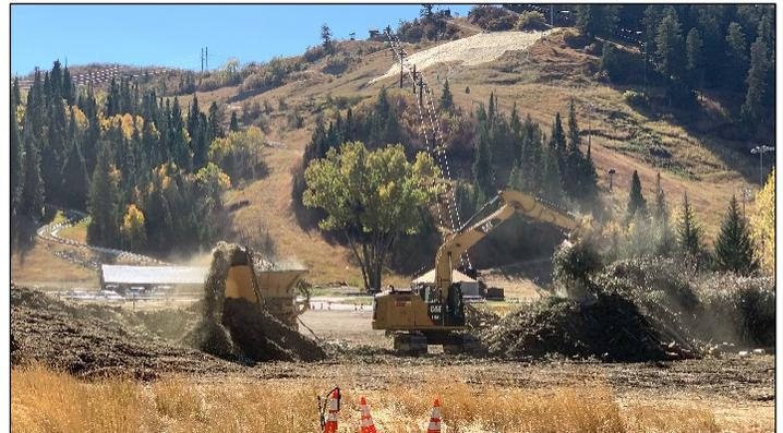
The city brought in a Vermeer Colorado TG5000 tub grinder to tackle the mountain of limbs, branches and stumps. This specialized machine provides powerful processing through a 540 horsepower Caterpillar engine and spinning duplex drum that pulverizes the material.
