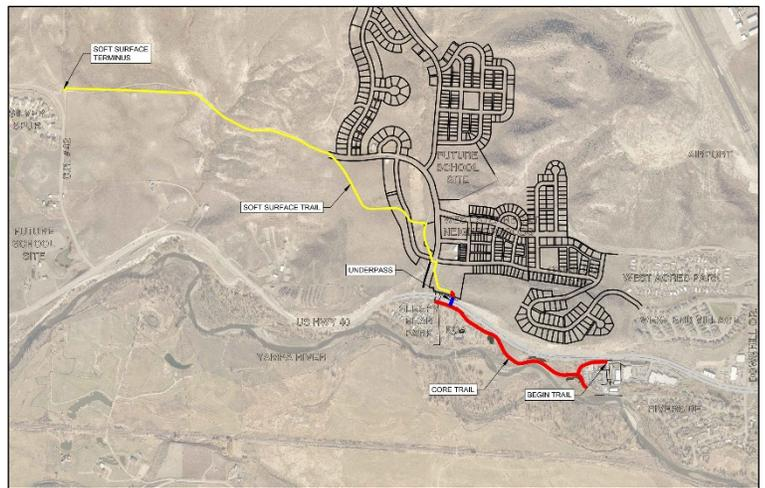
The design includes multimodal facilities totaling 2.17 miles linking residents in the neighborhoods on the westside of Steamboat to the overall pedestrian and trail network. The design includes approximately 800 feet of 8-foot hard surface sidewalk, 2,750 feet of 10-foot-wide hard surface Core Trail with 3-foot soft surface trail edge along Highway 40, 8,000 feet of soft surface trail, and a separated grade crossing of the state highway.
