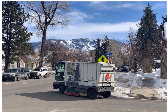
The city utilizes two very different sized machines in its sweeping arsenal. The smaller Sentinel Sweeper is an all-season street sweeper while the larger TYMCO DST-6 Regenerative Air Sweeper is a heavy-duty powerhouse with twice the capacity. Both vehicles collect heavy dirt, sand, gravel, and scoria and can follow the contours of uneven road surfaces in dry or wet conditions.
